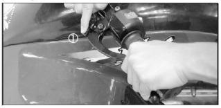
1.Rear brake lock plate(The rear brake is drum brake)
