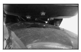
2. Remove the bulb holder cover, remove the bulb holder screw and the defective bulb.
