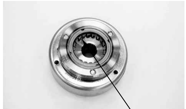
Starter One-way Clutch
