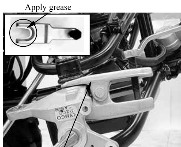
Ball Joint Remover
